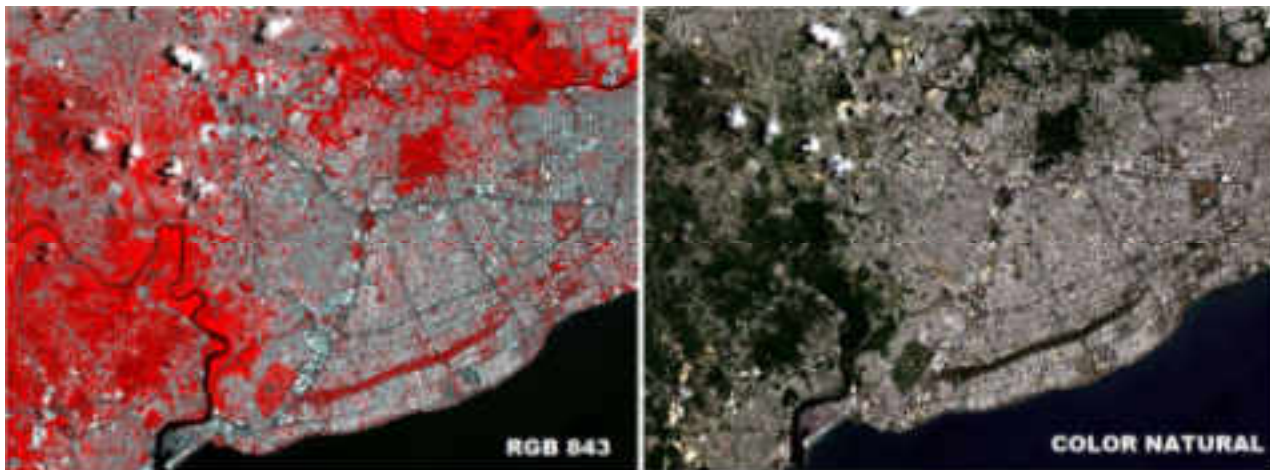
Figure 6-15: Images from Remote Sensing processing to determine Runoff Coefficient
