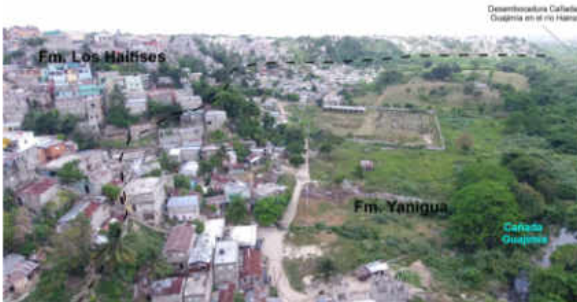
Figure 6-1: Boundary of the Yanigua and Los Haitises Formations in the Downstream Area of the Guajimía Canal
