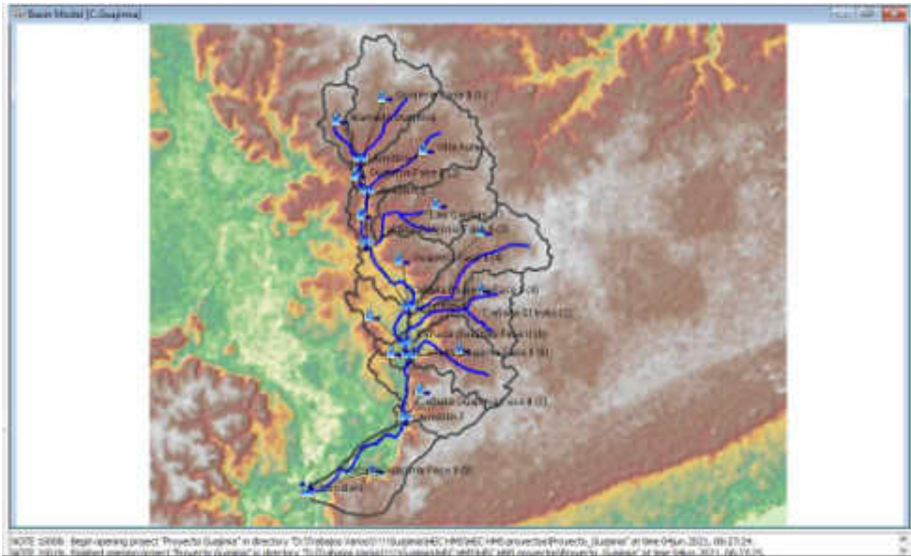
Figure 6-16: Example of Computational Node Mesh for the Calculation of Hydrometry in the Guajimía Canal
