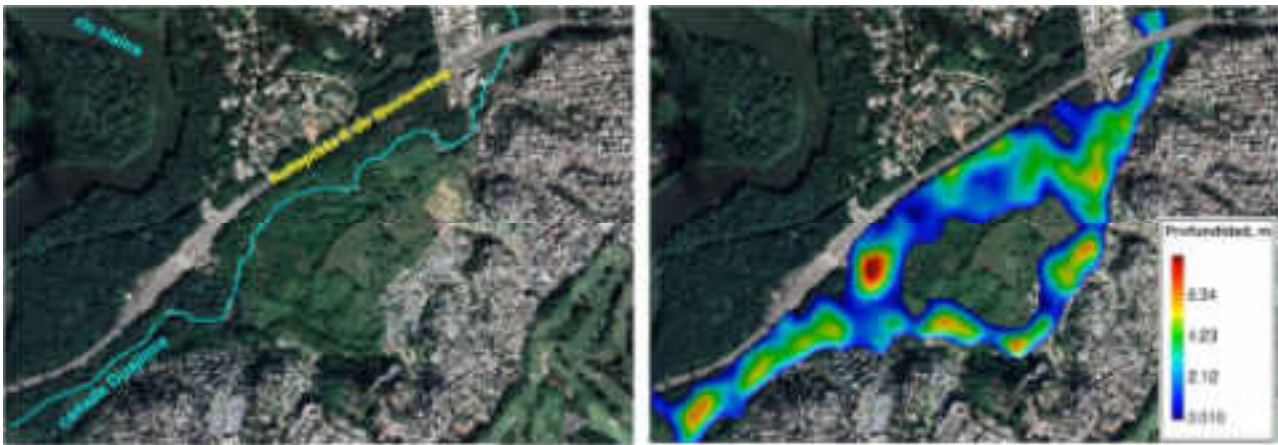
Figure 6-20: Estimated Flood Conditions in the Lower Third of the Guajimía Watershed, due to the Occurrence of Extreme Regional Rainfall
